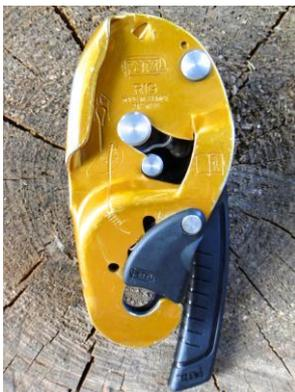
Should climbers wish to use this device on a single, stationary line without a back-up, they will be required, based upon rule 2.2.12, to disable the black plastic safety gate on the RIG and the I'D S by inserting a suitable rivet or bolt into the slot indicated by the red arrow, (See images) thus preventing unintentional opening of the device.
